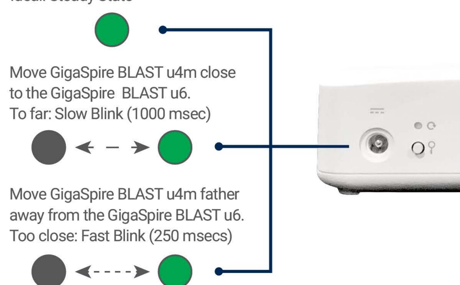
**Note:** Once successful pairing is complete, the GigaSpire BLAST and GigaMesh LEDs will both show a solid cyan (light blue) colour. It may take several minutes to reach this state.
